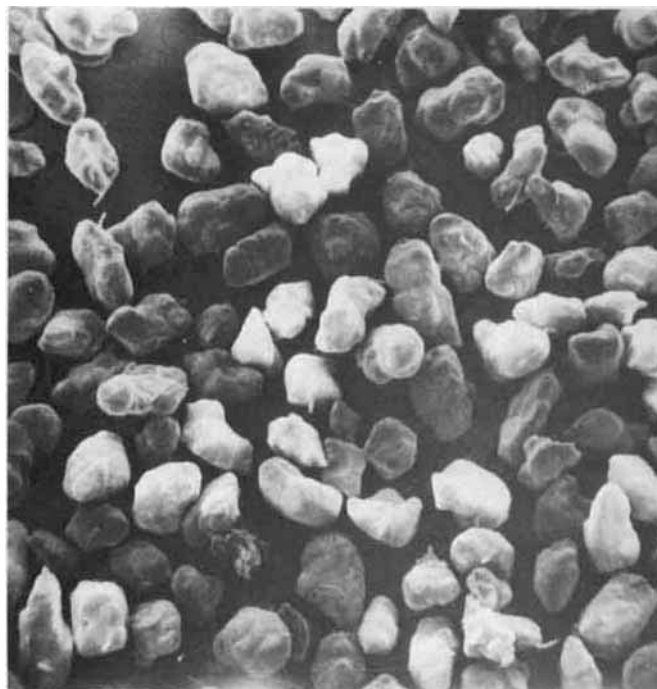
Figure 4 —Scanning electron micrograph of salicylamide microcapsules (see text).
